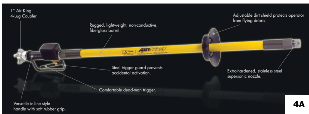
Figure 4A: Air Spade for use in the Compressed Air Soil Displacement Process
